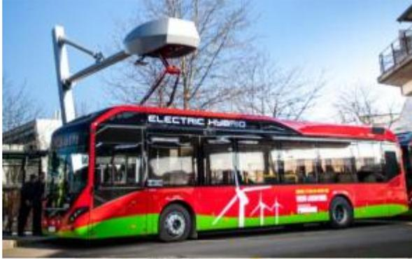
Drop down Pantograph
