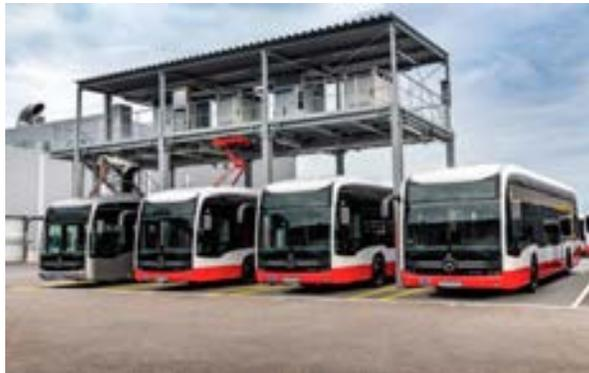
Bus Mounted Pantograph
