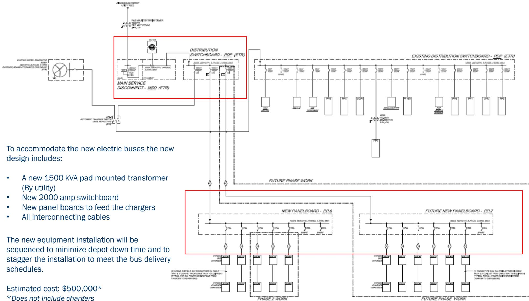
To accommodate the new electric buses the new design includes:
