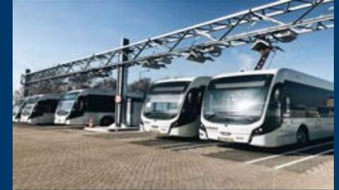
Roof Mounted Pantograph
