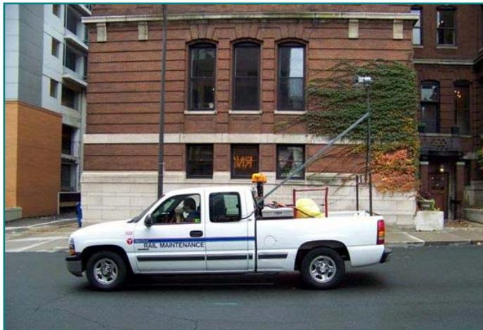
Engineers put a Hiawatha LRT horn and bell system on the back of a pickup to test noise impacts to Cedar Street buildings.
