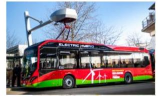
Drop down Pantograph Utilized heavily for on-route charging in the US.
