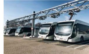
Bus Mounted Pantograph Utilized heavily for on-route charging in the Europe. First Pantograph Indoor charging System In Europe.
