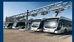
Roof Mounted Pantograph
